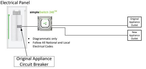
b. The **simpleSwitch 240<sup>™</sup>** can be teed in downstream of the panel at a point that requires the least amount of fishing, demo and wall repair.
